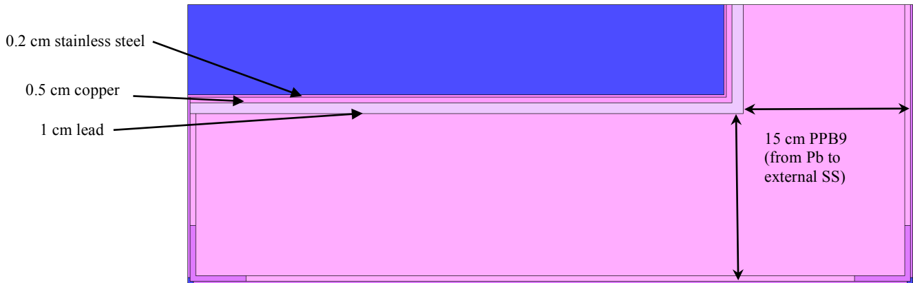
Figure 3-9. Internal Material Layers of Collimator Model (blue is air).
