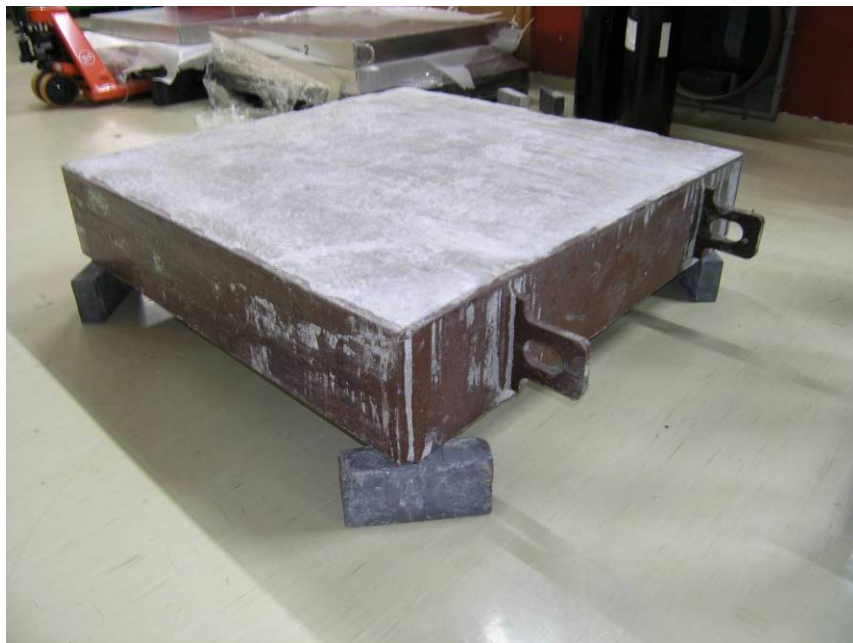
Figure 1-25. Concrete Shield Block.
