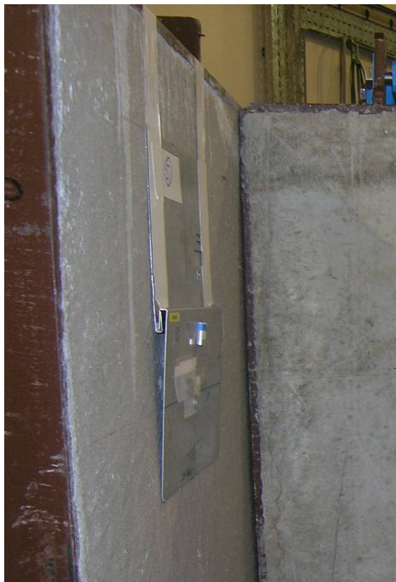
Figure 1-50. Plates Mounted in the Scattering Box.
