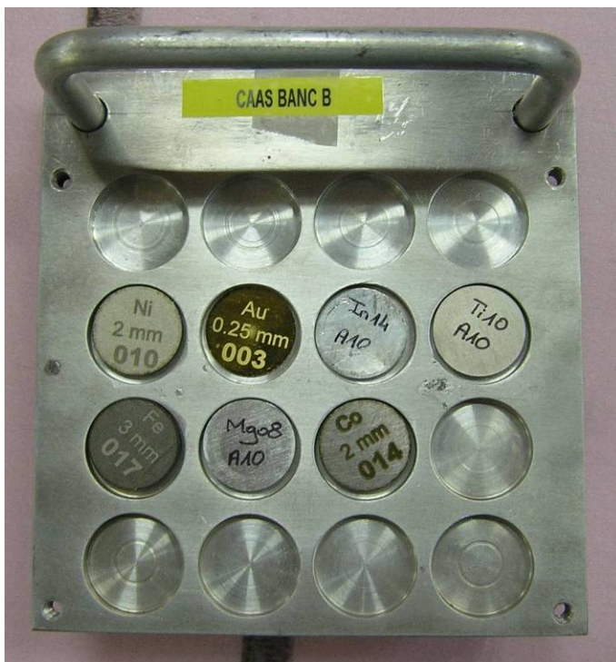
Figure 1-28. Collimator Foil Holder with Neutron Activation Foils.
