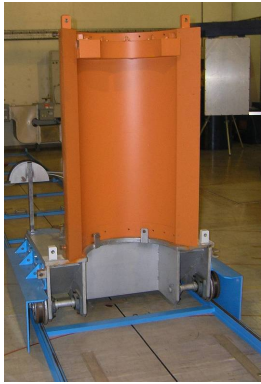
Figure 1-57. SILENE Lead Reflector/shield.
