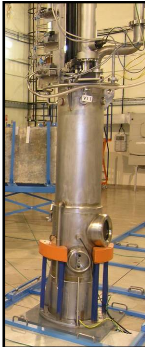
Figure 1-54. SILENE without the Lead Reflector.
