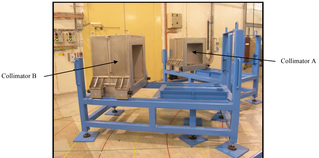
Figure 1-9. Collimators A and B on their Stands (without concrete shielding).
