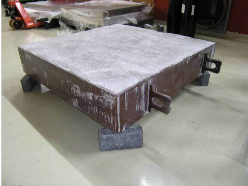
Figure 1-36. Concrete Shield Block.
