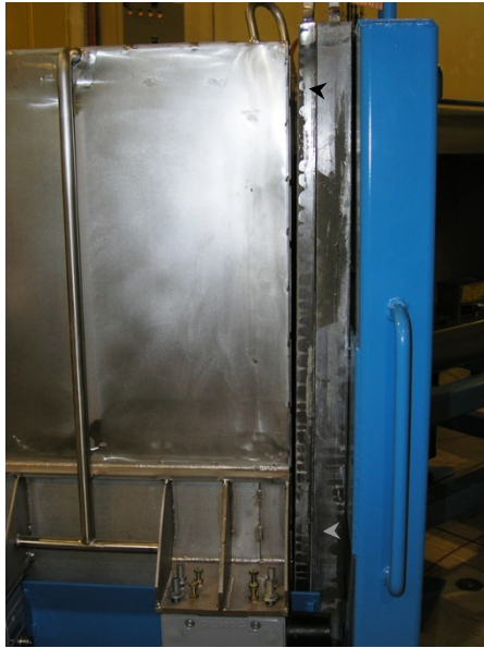
Figure 1-24. Collimator B, BoroBond Shield Blocks, and 1.5 cm Gap.
