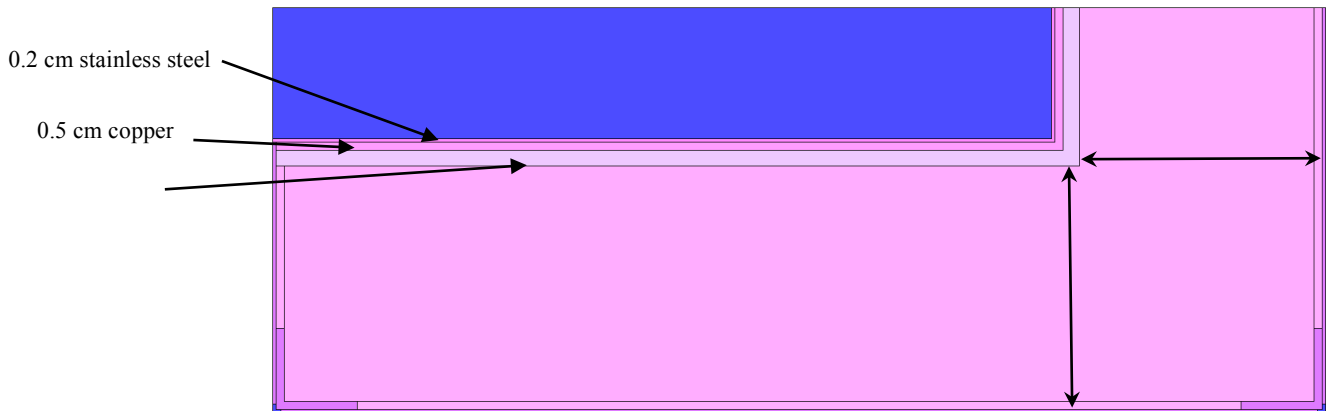
Figure 3-9. Internal Material Layers of Collimator Model (Blue indicates Air).
