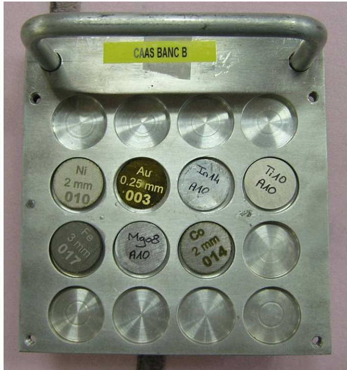
Figure 1-28. Collimator Foil Holder With Neutron Activation Foils.
