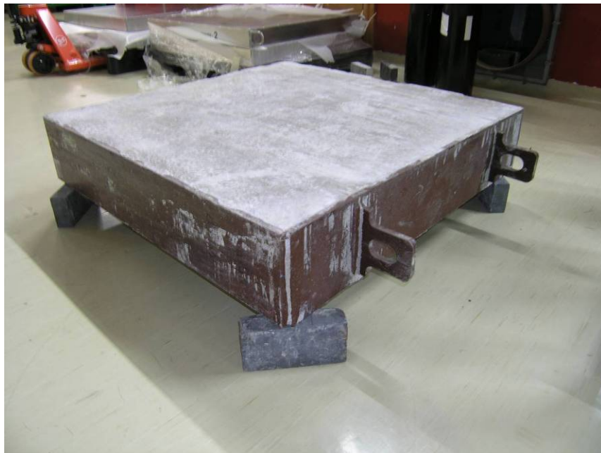
Figure 1-25. Concrete Shield Block.
